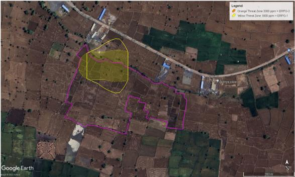
When, flammable chemical escaping from tank chemical is **NOT** on fire Choose Hazard to Analyze: **Blast Area of Vapour Cloud Explosion**
