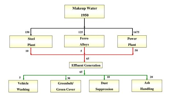
Figure 4 Water Balance Diagram
