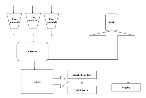
Figure 2 Process Flow Diagram (Ferro Alloys)
